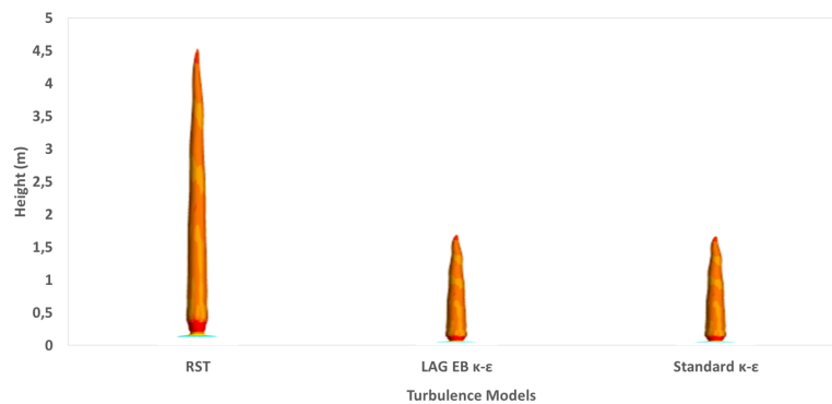
Figure 3.7: Predicted flame height for the three turbulence models
