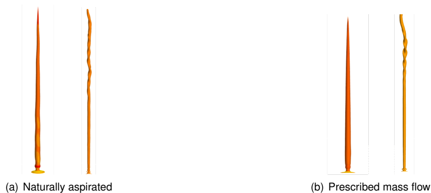
Figure 4.3: Predicted isosurfaces for mixture fraction and Q-criterion
